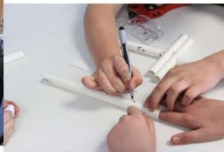
Measuring parts for the Sea Perch Robot frame.
